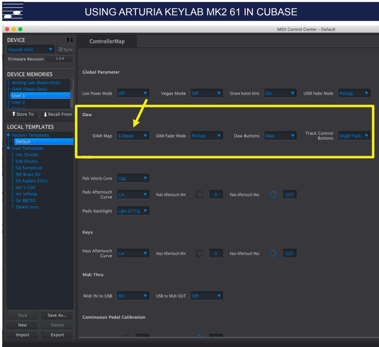
The former is the regular port when the keyboard as used for MIDI note input; the latter port is relevant when controlling the DAW with the KeyLab elements such as faders, knobs and buttons.
